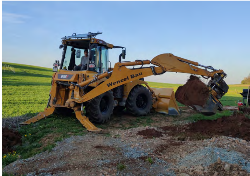
With the 280 degree slew range, the material can also be loaded on the side.
