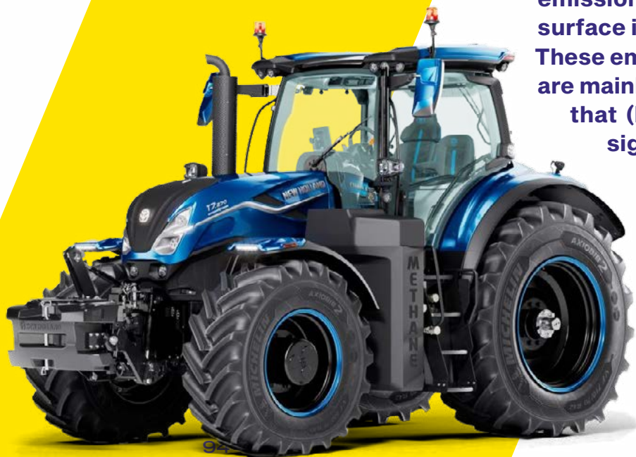
New Holland T7 Methane Power LNG: The first LNG tractor prototype Image source: New Holland
