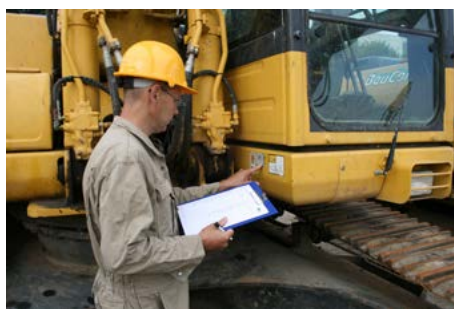
A record of the machine's condition is an integral part of the inspection Image source: MEVAS
