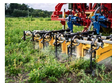
The Weed Control System detects and eliminates weeds organically with high precision Image source: Continental
