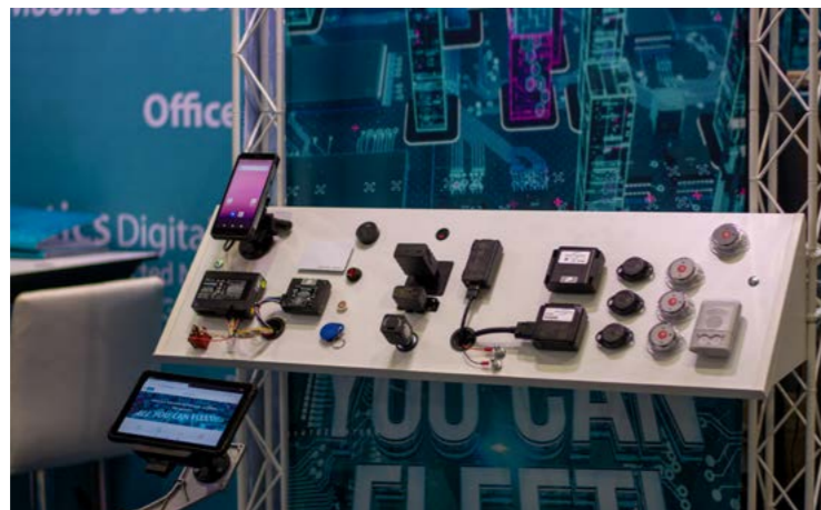
AC hardware/demo board: Retrofit telematics for all the equipment of a construction company (trucks, cars, vans, machines, trailers, containers, tools, etc.) Image source: AREALCONTROL
