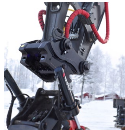
QuickChange™ allows excavator operators to change hydraulic attachments without leaving the cab.
