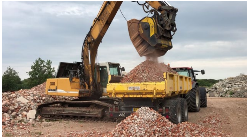
BF90.3 crusher bucket mounted on Liebherr 914
