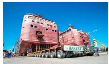
Hareket Heavy Lifting & Project Transportation won the contract to move two 6,200 t passenger ships over a distance of 250 m to a floating dock at the Tersan Shipyard.
