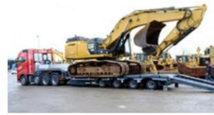
**NOOTEBOOM SEMI LOW-LOADER WITH HYDRAULIC WIDENING**
