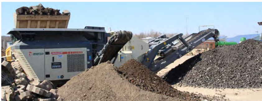
Metso Nordtrack J90 mobile crusher
